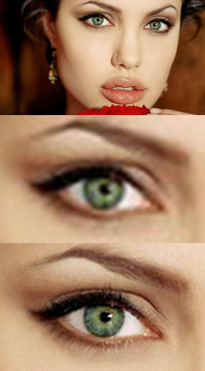
Fig.2: Image interpolation using linear method of interp2 built-in MATLAB® function. Top: original image. Medium: close-up of eye in image. Down: interpolated image.
